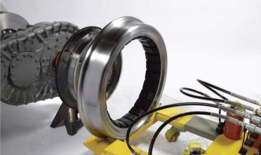
This conical ring still has jacking bolts in-place after the ring's removal. Remove and retain jacking bolts for later use.
