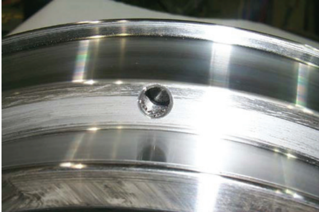
A damaged 1/2"-20 TPI hole in a Bochum 84 Wheel Center.
