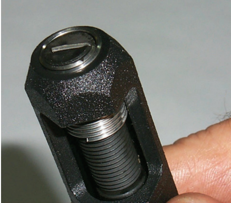
View showing a Heli-Coil inserted into the tool. Note that the tang of the Heli-Coil is in contact with the driving contour of the mandrel.
