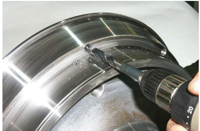
Drilling out the damaged hole using the provided 33/64" dia. drill bit.
