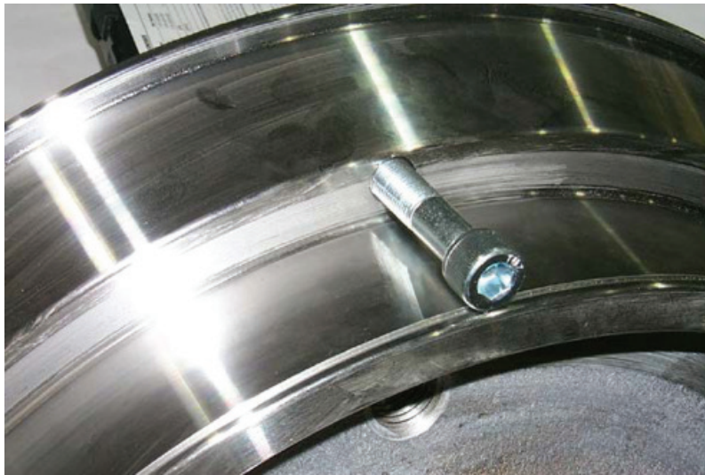
Test the threads with a 1/2"-20 cap screw.
