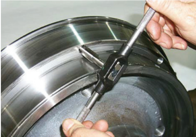
Start tapping without an extension for control.
