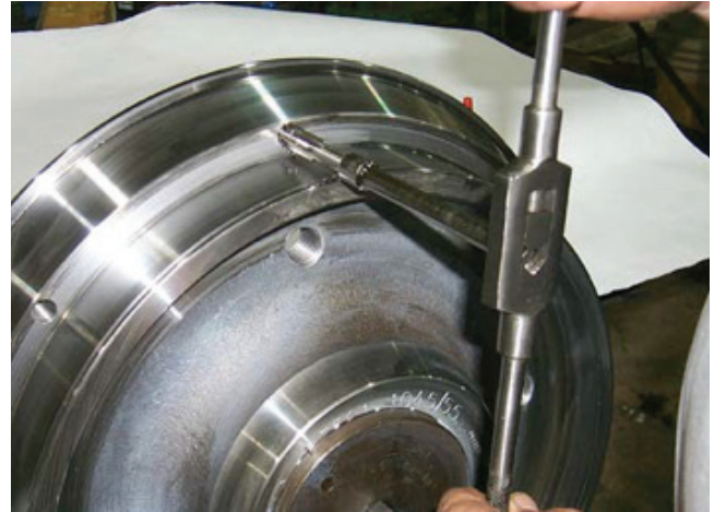
Use an extension to clear the wheel center face.
