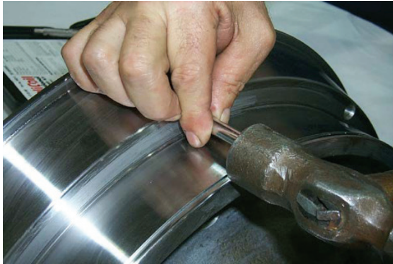
Using the steel rod (supplied with kit) to remove the tang from the Heli-Coil.
