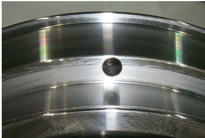
Re-drilled hole ready for tapping.
